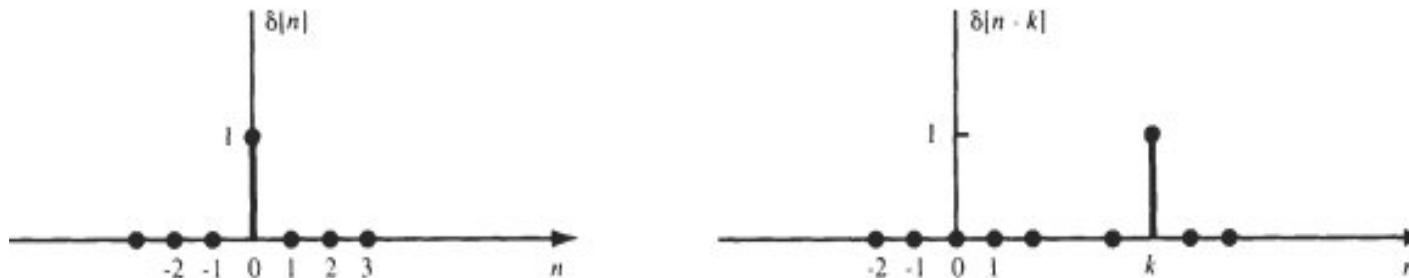
Fig. ( a )Unit impulse (sample) sequence; (b) shifted unit impulse sequence.
