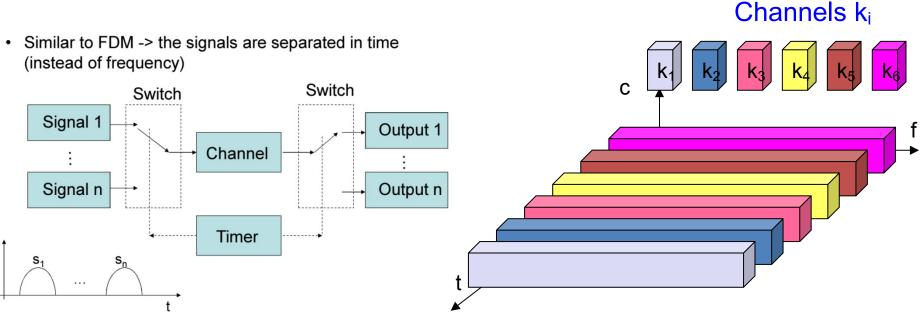
TDM is a **digital multiplexing technique** for combining several low-rate digital channels into one high-rate one. Channel gets the whole spectrum for a certain amount of time. Advantages: only one carrier in the medium at any time throughput high even for many users but the disadvantages the precise synchronization necessary Time division multiplexing can be applied to sampled analog signals directly or accomplished at the bit level
