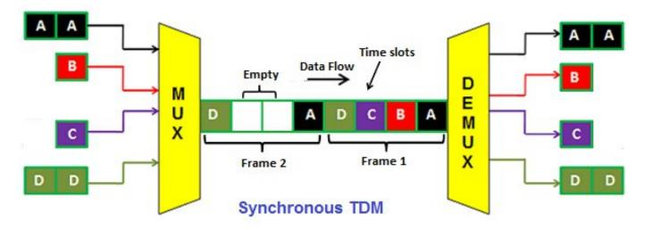
As shown in the below figure, the various time slots are arranged into frames and each frame consists of one or more time slots dedicated to each device (transmitter). For example, if there are 3 devices, there will be 3 slots in each frame. Similarly, if there are 5 devices, there will be 5 slots in each frame.
